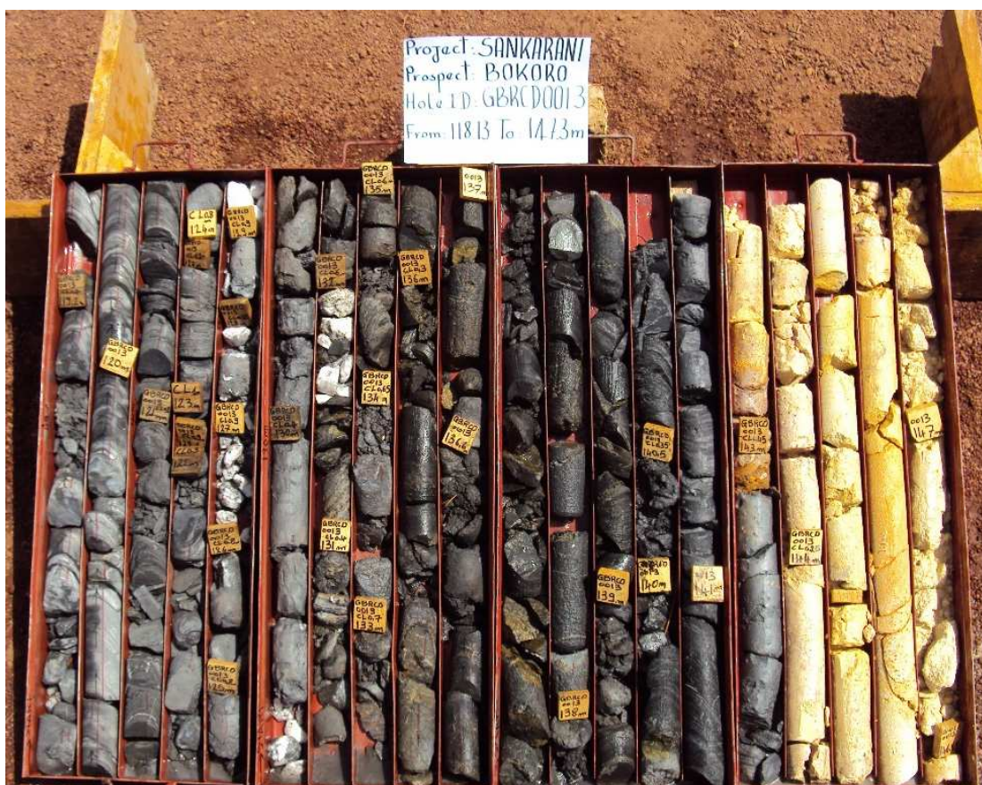
Figure 3-4: Poor quality fresh rock transitioning into highly altered rock
